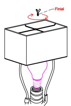
4. After inserting the lamp shade (P2) to U-shape brass harp and lock by Finial.
