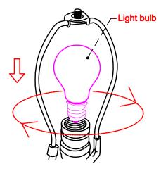
3. Install the light bulb by turning it clockwise.
