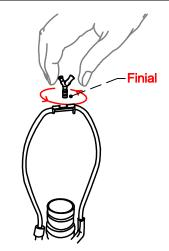
2. Remove the brass finial by turning counterclockwise.
